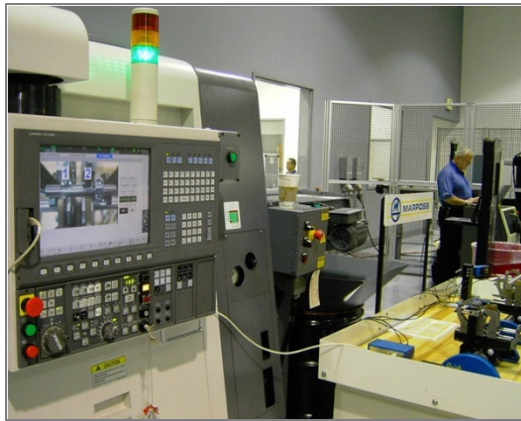
Marposs gage connected to LU300 via USB. The THINC®-OSP control screen provides operator guidance for gauging procedure.
